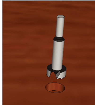
Drill or water-jet a 17mm-diameter hole.
